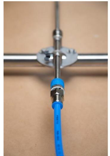
Detach the crossbar from the locking mechanism and lift it out of the container. Using a suitable material, clean the mixing lance by wiping it from the top down. Follow the operating instructions for the respective medium.
