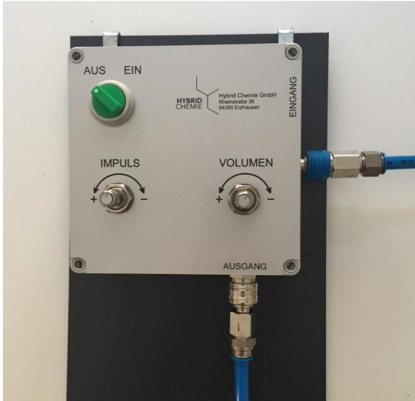
Now connect the compressed air hoses, and ascertain that they match the feed and discharge connections.
