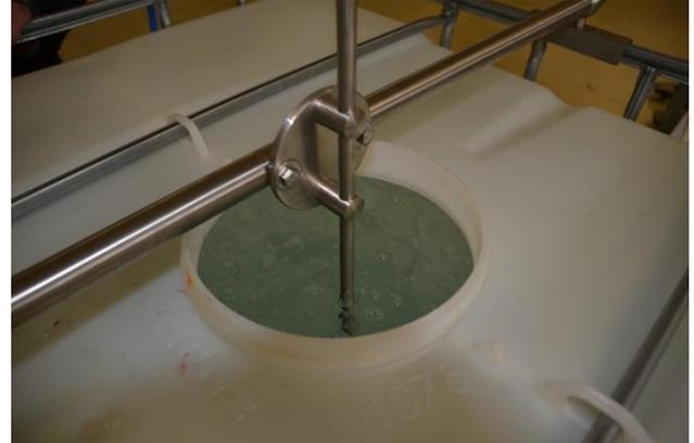
After inserting the mixing lance into the container, it must be locked in place. Using the left and right wing nuts, attach the cross beam to the metal cage of the container.
