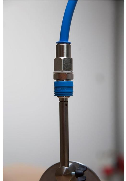
Open the compressed air feed line and adjust the pressure to 8 bar maximum. Ensure that a minimum of 400 L/min. intake air is available. Set the main switch of the control unit to “ON.” Adjust the control valves to minimum settings by turning them clockwise. The output capacity of the mixing lance can be varied individually by adjusting the two control valves (pulse, bubble volume). Once the desired settings have been obtained, use the locking screw to fix the control valves in position.
